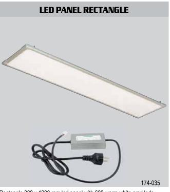
Rectangle 300 x 1200 mm led panel with 600 warm white smd leds. 50 Watt, 3350 lumen. Led driver included.
